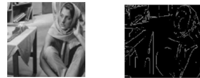
Fig.3. Image processing (a) After Averaging Template (b) After Averaging and Edge Detection
